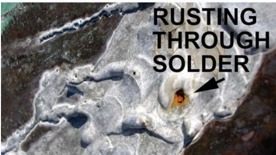
Figure 29: Copper rivets with steel mandrels will rust almost immediately, even through a solder joint.
