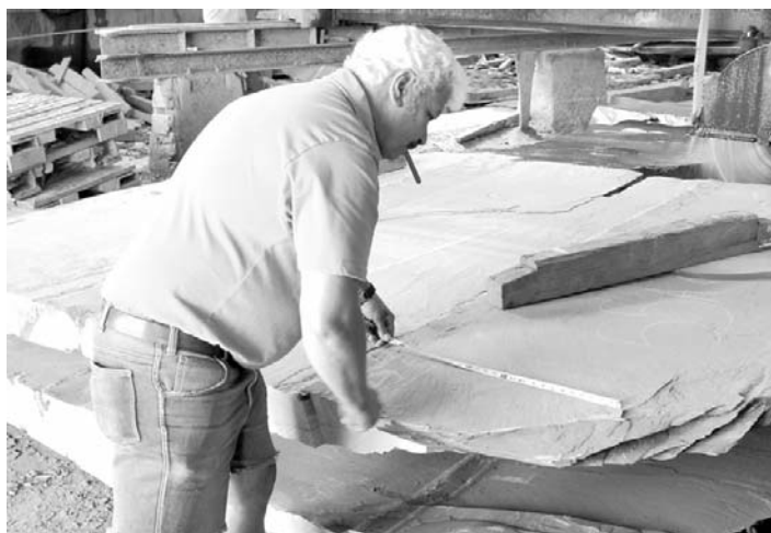
Pete Papay, president of the corporation at Penn Big Bed Slate Company, grades and marks a slate block in preparation for cutting with a diamond saw.
