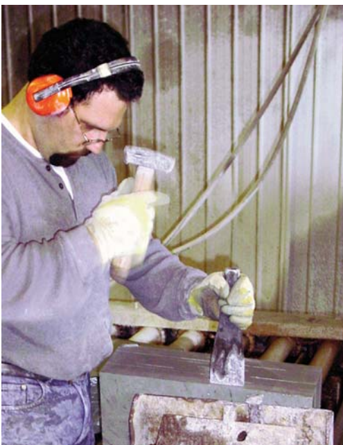
Shawn Camara, Vermont's most eligible bachelor, splitting a slate block into roofing slates at the Blissville Quarry.
