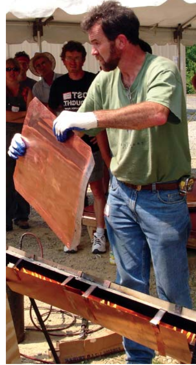
Barry Smith pre-tins copper pans in a pre-tinning trough.
