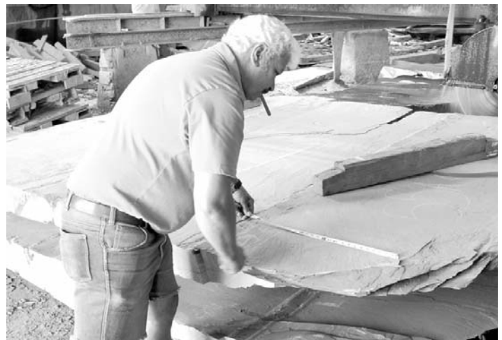
Pete Papay, president of the corporation at Penn Big Bed Slate Company, grades and marks a slate block in preparation for cutting with a diamond saw.
